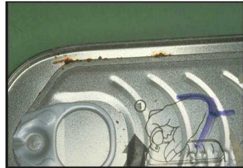
Damage to score-line (rusting from leakage)
