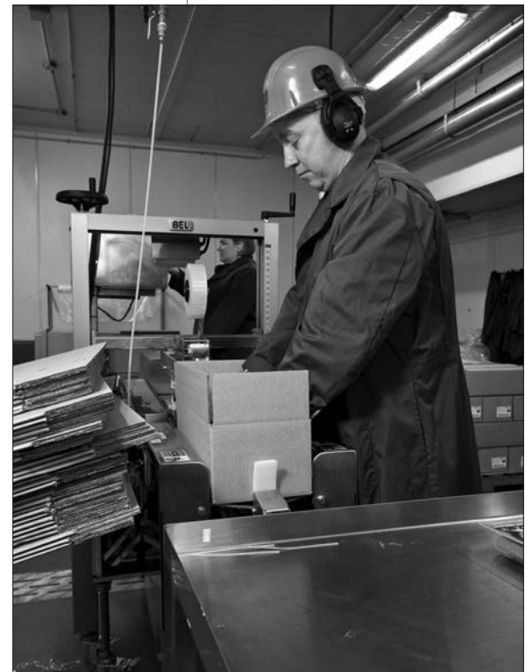
Hearing protection devices such as earmuffs are an easy, effective way to protect against exposure to hazardous noise levels.
